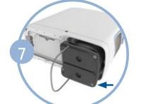
Remove the columns completely from the Inogen One<sup>®</sup> G5. Both columns are removed as one piece.
